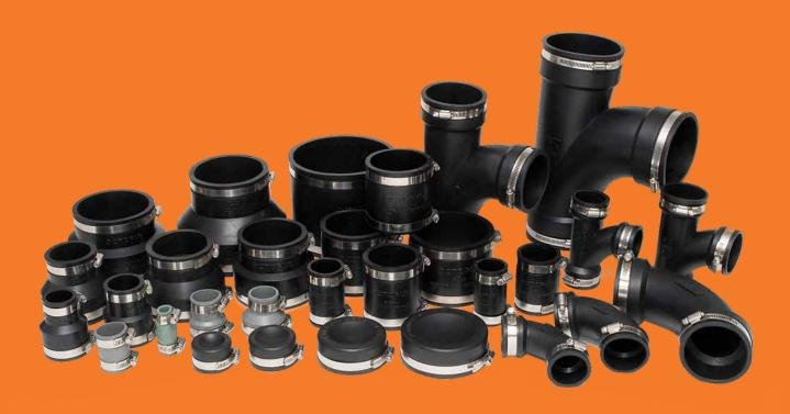
Octopus Plumbing has launched a wide, new range of metal banded flexible couplings to help solve many common plumbing problems. All couplings are fully AS/NZS 4327 approved. They are constructed from Type A PVC and are fitted with stainless steel hose clamps (316SS) so they are ready to go. All the common domestic pipe sizes are covered, from 32-150mm. The large range consists of regular PVC couplings, plus adapter couplings, clay couplings, tees, elbows, caps and more.
